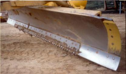
Potential solutions: carbide cutting edges or bits.
