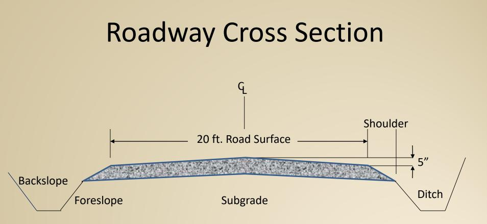
Generally recommended crown for gravel surfaces is 4% (1/2 in. of crown per foot) which is double the crown used in pavements.
